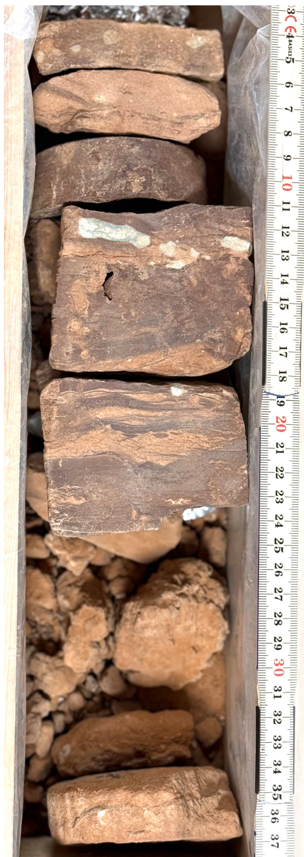
Fig. 11. Interval 1367-1373 m (4486-4506'), Volpriehausen Member, sandstone unit.
