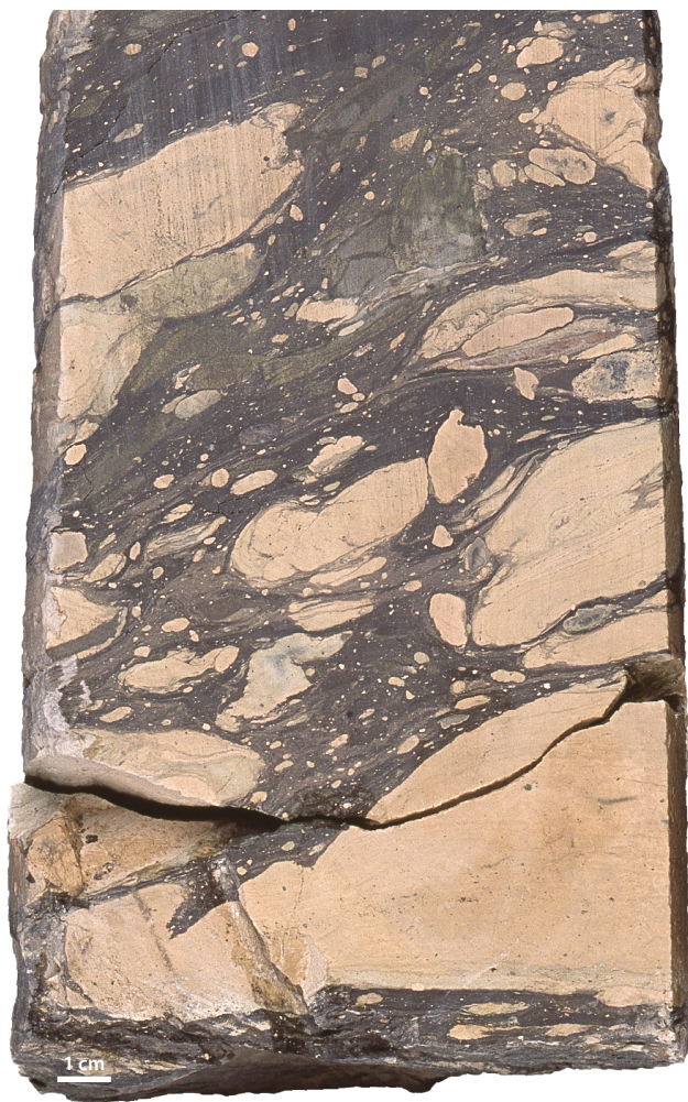
Fig. 13. Representative photograph of matrix-rich conglomerate (sedimentary structure e) in the Deep Adda-1 core (2446.25–2446.05 m), showing a marlstone-dominated (F5e), relatively chaotic and low-angle oblique fabric that contains dispersed granule to cobble-sized, plastically deformed chalk clasts with lenticular and elongated to contorted shapes and slight lamina convolutions.
