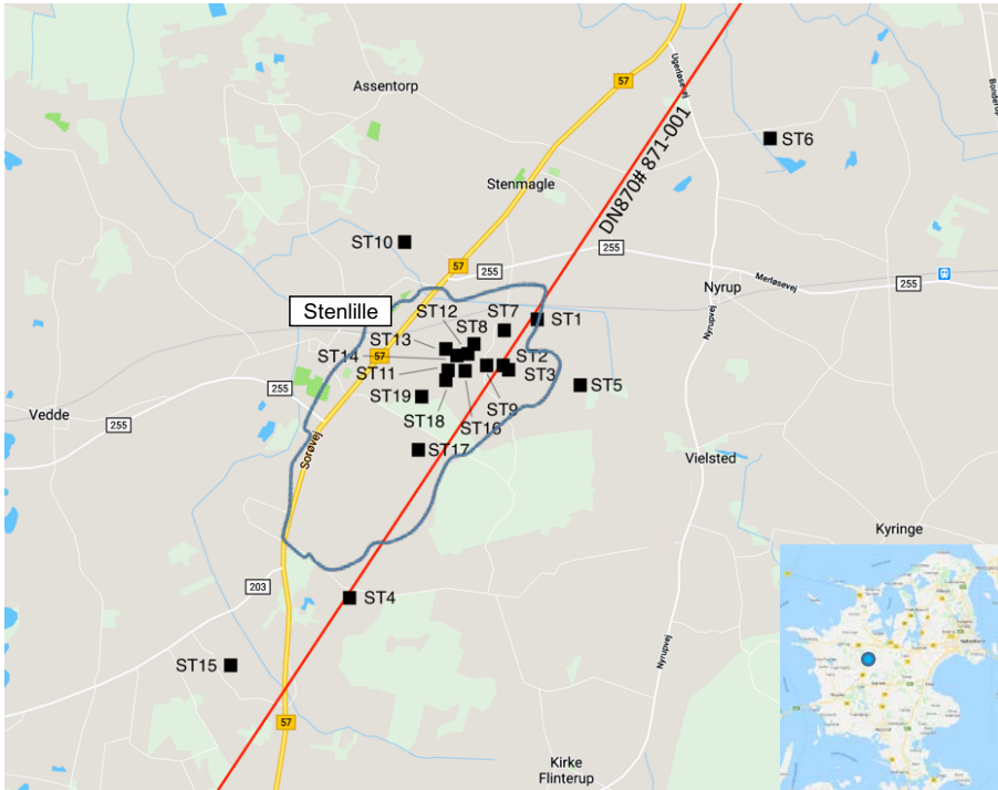
Fig. 1. Map of the Stenlille area on Sjælland with outline of seismic line DN870# 871-001 (shown in Fig. 2) and location of wells (black squares). The blue closed curve outlines the gas-bearing aquifer storage site. The yellow curve is a highway.
