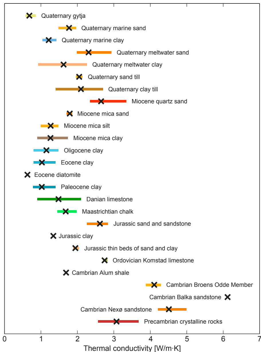
Fig. 8. Thermal conductivities for litho-chronological groups with decreasing stratigraphic age upwards. Crosses indicate mean values and colour bars show the range of measured conductivities. Colour code as in Fig. 2.
