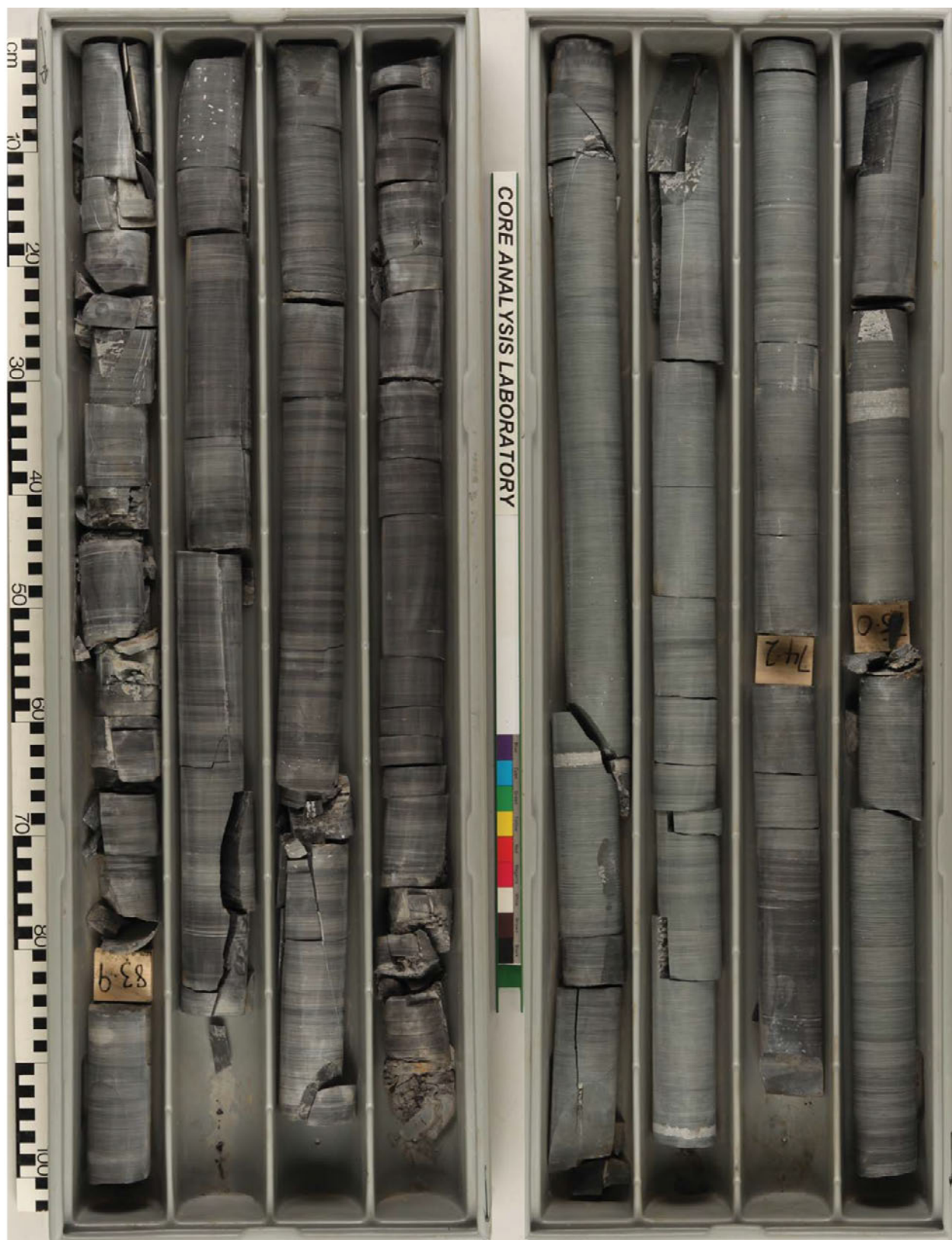
Fig. 5. Sommerodde-1 core boxes 22 (left) and 19 (right). Core box 22 (83.15–86.60 m) is entirely within log stratigraphical unit G1. Graptolites from the lower part of the Oktavites spiralis Biozone (Telychian) occur between 83.75 m and 84.38 m. Core box 19 (71.80–75.45 m) is entirely within log stratigraphical unit G2, dominated by greenish grey mudstones, of middle Oktavites spiralis Zone (Telychian) age.
