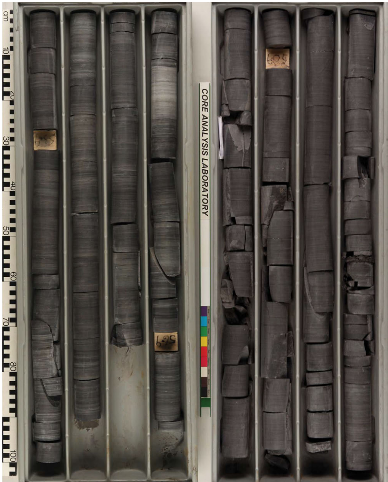
Fig. 6. Sommerodde-1 core boxes 14 (left) and 13 (right). Core box 14 (53.65–57.07 m) includes the boundary between log stratigraphical units G2 and G3, the base of G3 (at 56.4 m) marked by the base of the pale limestone. The highest Cyrtograptus lapworthi Biozone (Telychian) graptolites occur at 54.50 m. Above this level in this core box only long-ranging species were found. Core box 13 (50.10–53.65 m) is entirely within log stratigraphical unit G3, monotonous grey mudstones, with the lowest Sheinwoodian graptolite ( Cyrtograptus purchisoni ) recorded at 53.37 m.
