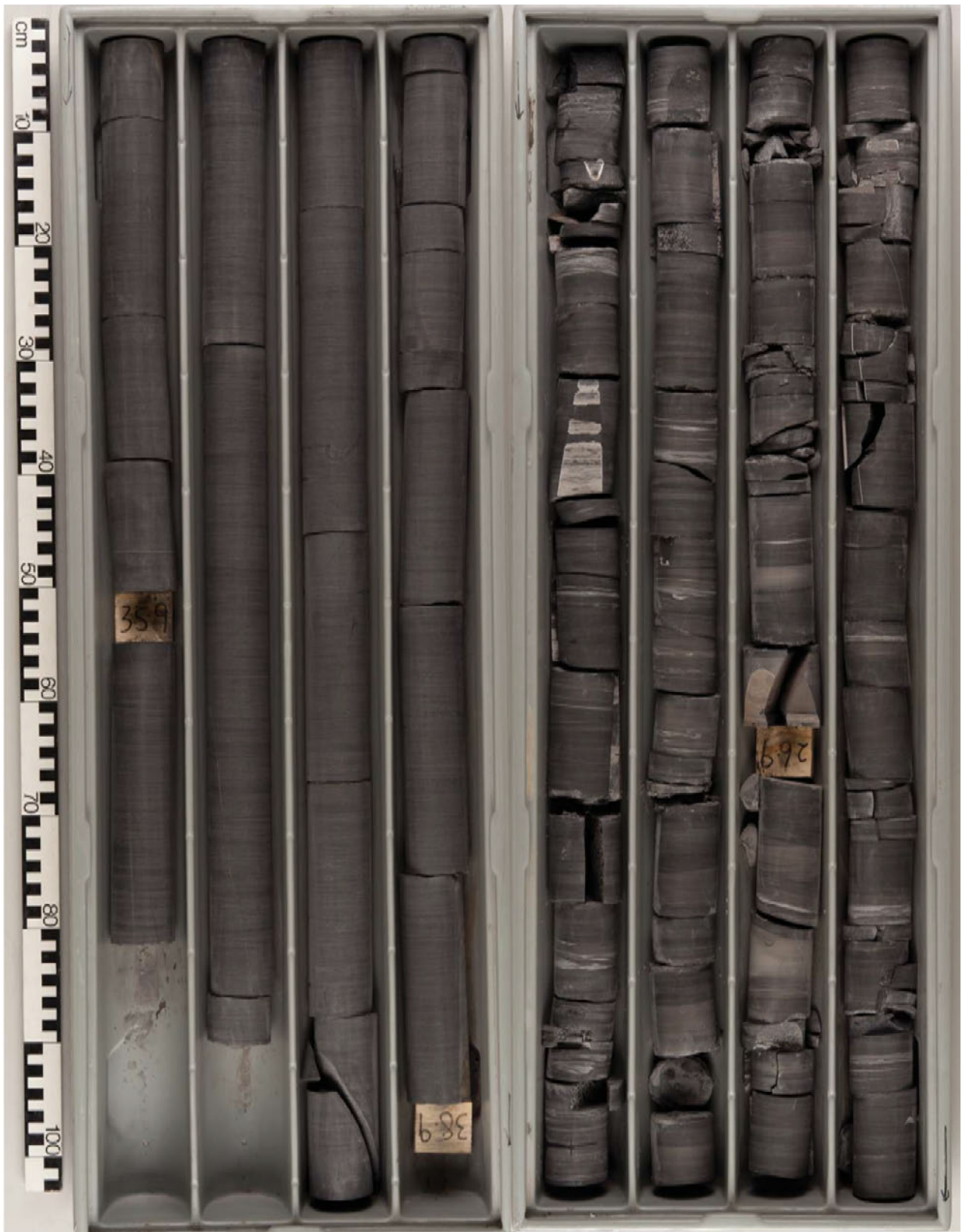
Fig. 7. Sommerodde-1 core boxes 9 (left) and 6 (right). Core box 9 (35.52–38.90 m) is entirely within log stratigraphical unit G4, monotonous dark grey mudstones. The base of the Monograptus riccartonensis Biozone (Sheinwoodian) is at 37.52 m. Core box 6 (24.50–28.20 m) is entirely within the lower part of log stratigraphical unit G5, interbedded siltstones/sandstones and mudstones. The core in this box is entirely of Cyrtograptus rigidus (late Sheinwoodian) age.
