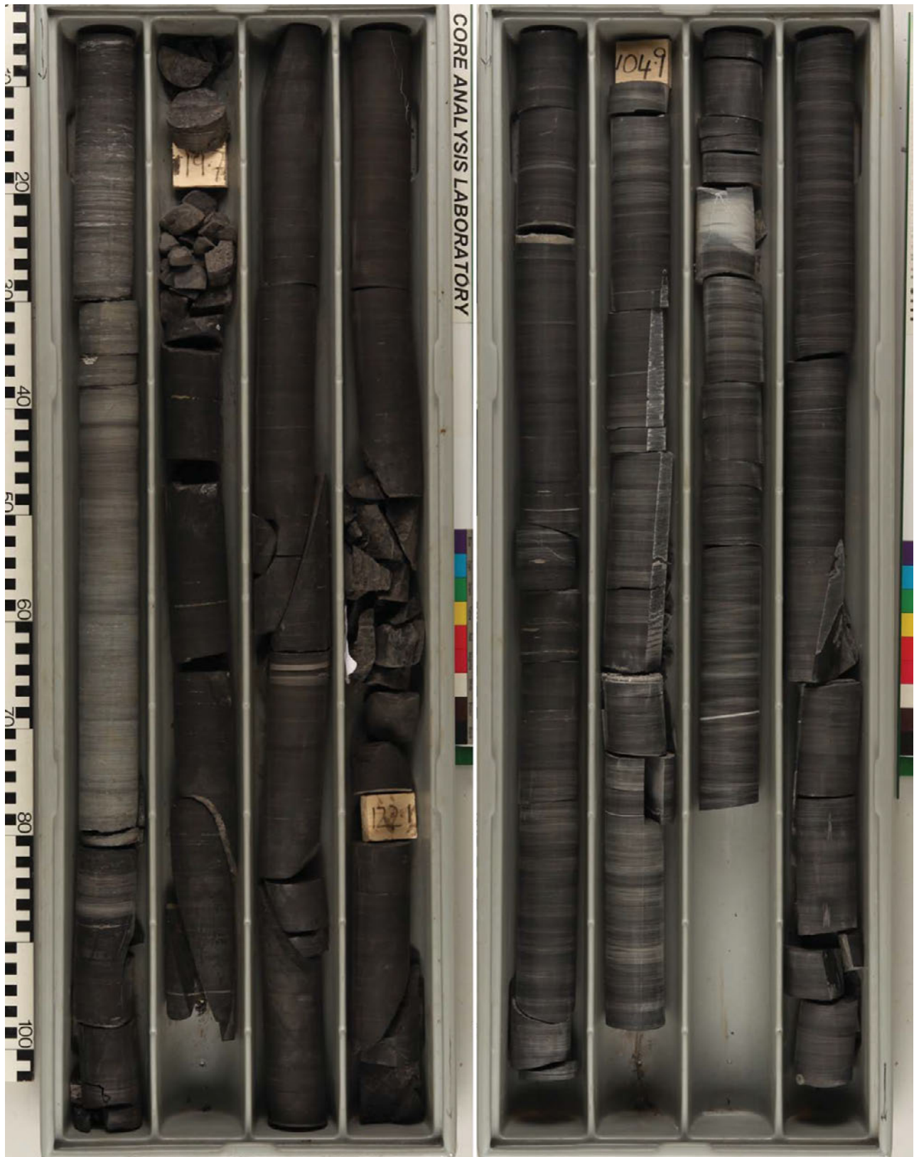
Fig. 4. Sommerodde-1 core boxes 32 (left) and 28 (right). Core box 32 (118.66–122.36 m) includes the top of log stratigraphical unit F4, comprising very dark mudstones of Lituigraptus convolutus Zone (Aeronian) age and the lowermost part of log stratigraphical unit F5 which consists of unfossiliferous grey silty mudstones. Core box 28 (103.93–107.40 m) is higher within log stratigraphical unit F5 and is entirely of Spirograptus turriculatus Zone (Telychian) age.
