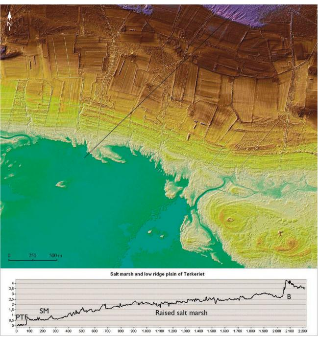
**Fig. 33.** Digital terrain model (DTM) of the Tørkeriet area in south-western Læsø (and Færøn, lower right) showing raised low-ridge plains (raised saltmarshes) between an older barrier (B) and the present saltmarsh (SM) fringing the pseudo-tidal flat (PTF). Levels of 35 beach ridges all 2–5 km long have been measured precisely along 381 transects each of 200 m length (Fig. 34).
