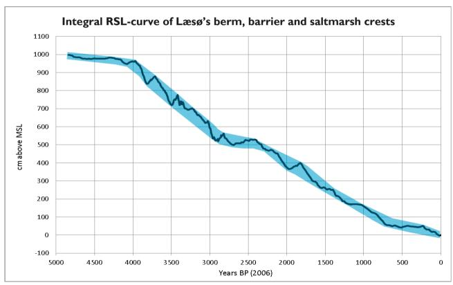
**Fig. 38.** Integral RSL curve of berm, barrier and saltmarsh crests on Læsø. The curve is detrended for height of swash and geological 'background noise' (Figs 32 and 35). Blue band: Limits of short-term sea-level oscillations. The vertical widths of the blue band indicate that the sea level oscillated many times within limits of 0.5–1.1 m of the general trend of the RSL curve, e.g. 0.6 m during the Little Ice Age lowstand between 850 to 200 years BP (1250–1800 AD).
