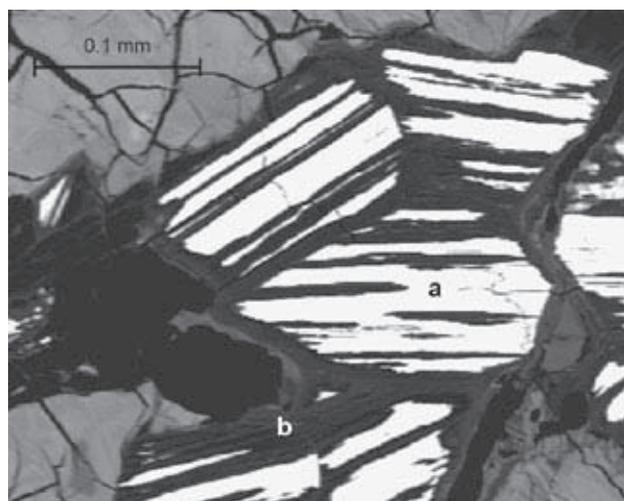
Fig. 4. Aggregate of chalcothallite/mineral X grains (a) partly decomposed to secondary phases (b, Tables 4-1 and 4-2).
