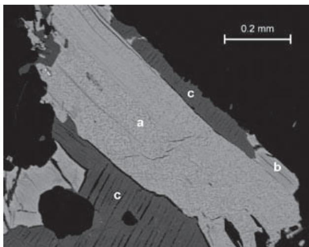
Fig. 3. A relatively large chalcothallite grain with the exsolved unidentified phase (a) in contact with chalcocite (c). On the extreme right a fragment of mineral X (b) lies in contact with chalcothallite and morphologically resembles the associated secondary ‘chalcocite’.
