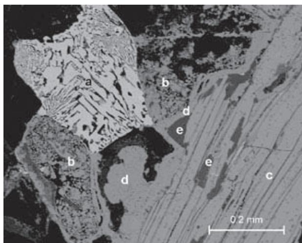
Fig. 10. Exsolution aggregate of antimonian silver (a) enclosed in decomposed cuprostibite grains (b) in contact with chalcothallite (c). The outline of the original cuprostibite grains is marked by a narrow layer of grains of antimony oxide (d). A primary phase (e) of the chalcosite group lies interstitial to chalcothallite.
