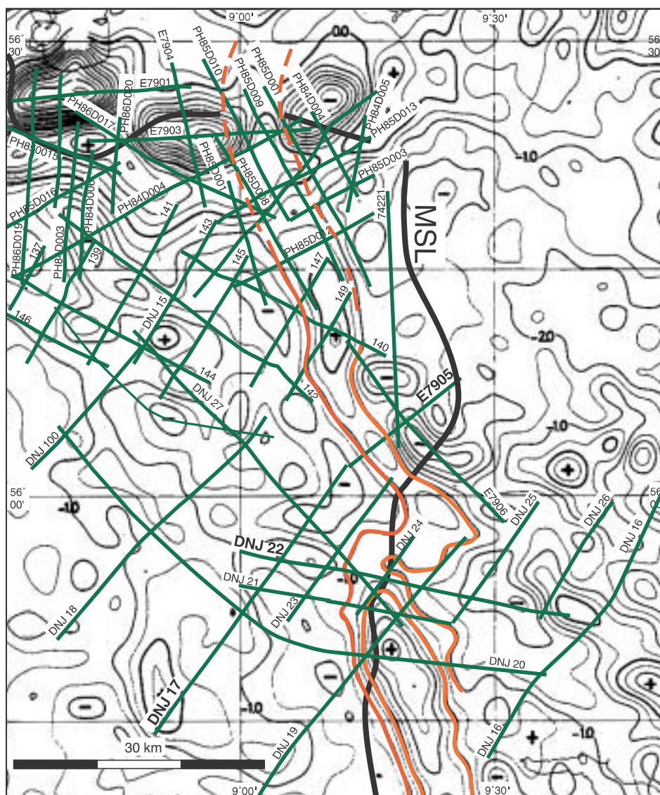
Fig. 6. Reflection seismic lines in the study area against the residual gravity anomalies. The limits of the N-S trending residual positive gravity anomaly are marked with red lines.
