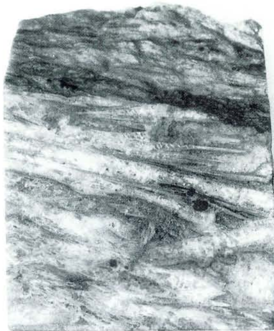
Fig. 2. Cut and polished section through a columnar aggregate. White patches are fine-grained strontian barite in jarlite. Lamellae are cut along their lengths. The area shown is 4 \times 5 cm.
