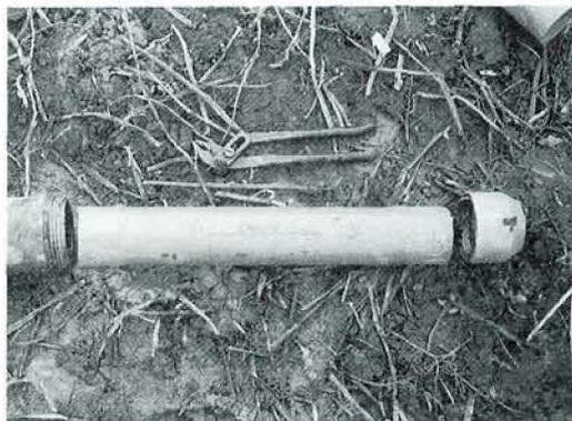
Fig. 3. Plexiglass tube with a till core disengaged from drilling device.
