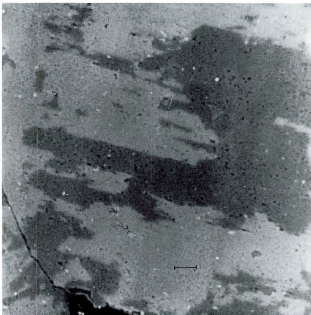
Fig. 3. Photo of the back scatter electron image of the microprobe. Dark grey albite, light grey potassium feldspar. Scale bar is 5 \mu\text{m}
