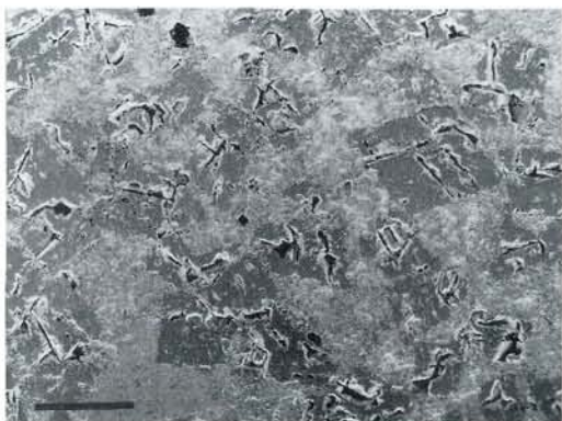
Fig. 5. Scanning electron micrograph of polished and etched section of partially dolomitized bryozoan limestone showing idiotopic-euhedral texture. The intercrystalline area is primarily filled by secondary calcite cement. Note dedolomitization along cleavage traces in the individual dolomite rhombohedra. Bar scale 100 \mu\text{m} .
