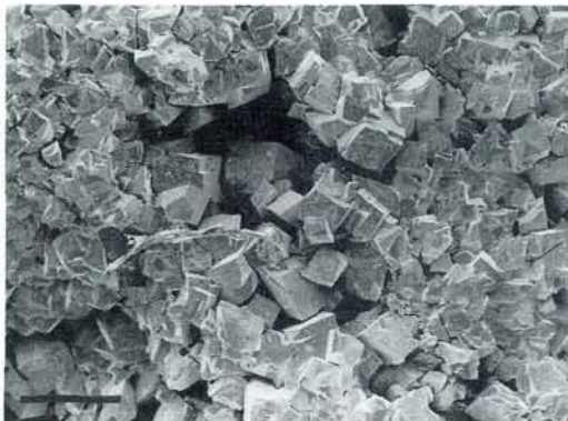
Fig. 3. Scanning electron micrograph of completely dolomitized bryozoan limestones showing idiopathic-subhedral to sucrosic texture. Fracture surface. Bar scale 200 \mu\text{m} .
