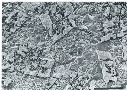
Fig. 10. Scanning electron micrograph of polished and etched specimen from the central part of a dolomite concretion showing variable dedolomitization in dolomite in dolomite rhombohedra. The intercrystalline area is filled by secondary calcite cement. Bar scale 100 \mu m.
