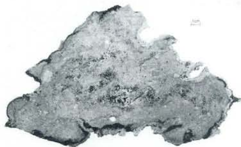
Fig. 9. Section of dolomite concretion from Fakse Quarry. Note the irregular outline and the outermost black rim which indicates iron oxides.
