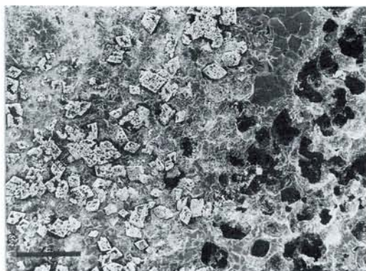
Fig. 12. Scanning electron micrograph of polished and etched specimen from the margin of a dolomite concretion. The dolomite rhombohedra (left) have been intensively dedolomitized and subsequent leaching has resulted in moldic rhombohedral porosity in the outside margin (right) Bar scale 300 \mu\text{m} .
