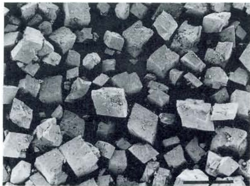
Fig. 4. Scanning electron micrograph of dolomite sand. Note that the sediment almost exclusively consists of dolomite rhombohedra. Bar scale 200 \mu\text{m} .
