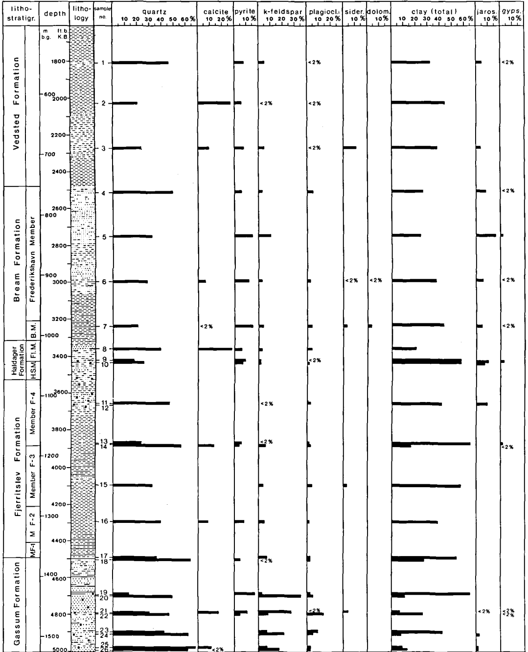
Fig. 4 & 5. Bulk mineral distribution. H. S. M. = Haldager Sand Member, Fl. M. = Flyvbjerg Member, B. M. = Børglum Member (The lithology is modified from Larsen (1966) and Michelsen (1978).)
