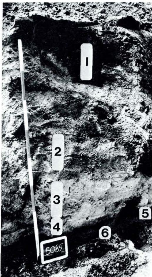
Fig. 7. Photo of profile at km 5.085 with wood fragments probably *in situ* (black part in right hand lower part of profile). (1) involuted fine sand, sand, and gravel, (2) medium sorted, 375 µm sand with a little gravel, dark ochre, fluvatile, (3) as (2) but gray-light ochre, (4) light gray, well-sorted, well to subrounded 105 µm sand, eolian, (5) as (4) but gray with small pieces of wood and faint bioturbation, (6) as (4). The topsoil is removed. The units of the ranging pole are 20 cm long.
