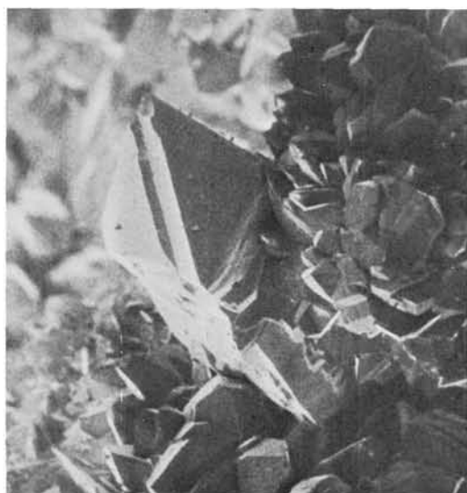
Fig. 3. Crystal of wulfenite, from the prosopite material, showing parallel growth. S.E.M. \times 150 .
