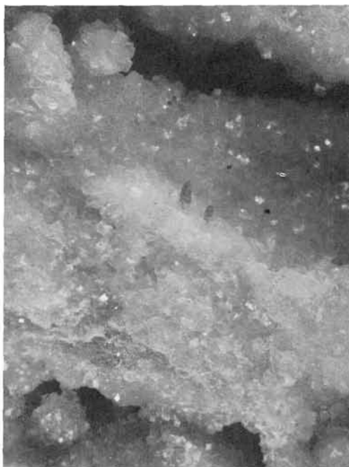
Fig. 4. Aggregate of cube-like crystals of thomsenolite, \times 1.5 .
