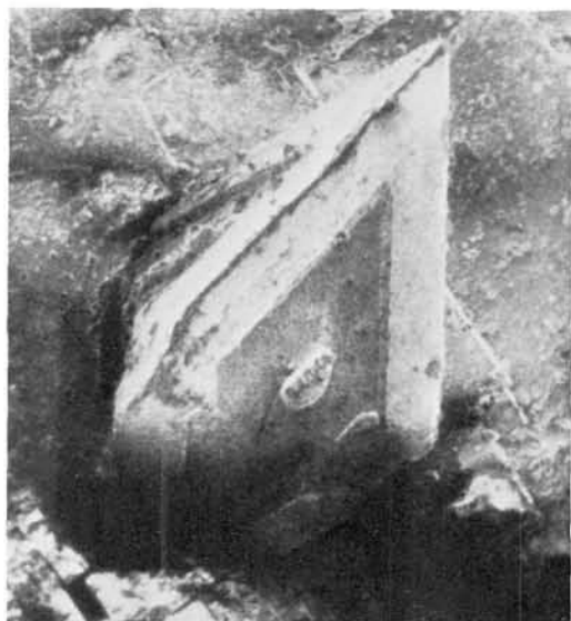
Fig. 5. Hopper crystal of wulfenite. S.E.M. \times 150 .
