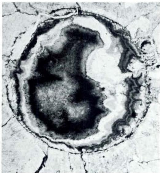
Fig. 5. Light micrograph of sectioned specimen showing zonation as well as supposed shrinkage phenomena. 85 x.
