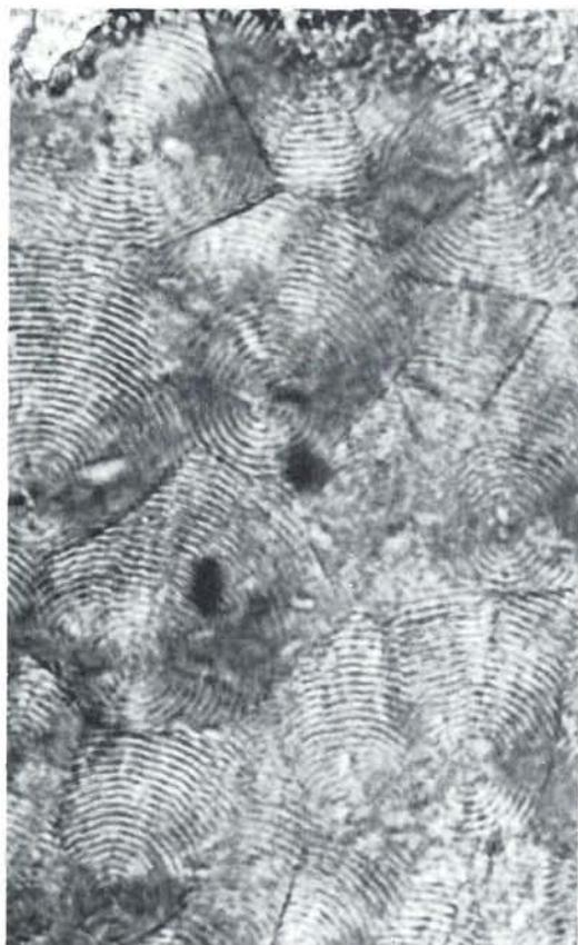
Fig. 17. Detail of specimen shown in fig. 15 but another area. Note poor definition of periodicity where twin boundaries are parallel with polarizer direction (north-south). 500 x. One nicol. LM.
