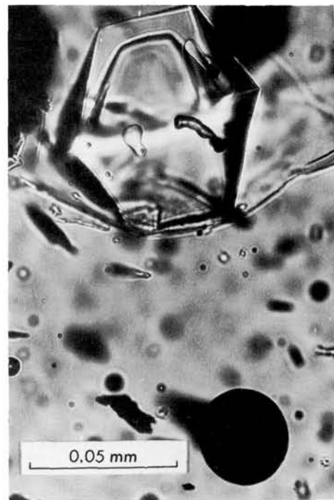
Fig. 6. Graphite-andesite glass with an euhedral phenocryst of olivine (top) and an immiscible sulphide-metallic iron sphere (bottom) similar to that shown in fig. 10. A few flakes in the glass are graphite. GGU 8034.
