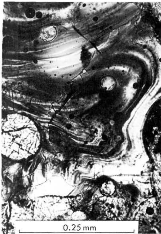
Fig. 5. Flow-folded, highly inhomogeneous glass, recording the initial stage of mixing of basaltic magma and liquid derived from the melting of sediment. Some of the tiny black spots are spheres of sulphide and iron, others are gas bubbles. GGU 5646, tuff layer no. 1. Analyses from this grain are shown in table 4.
