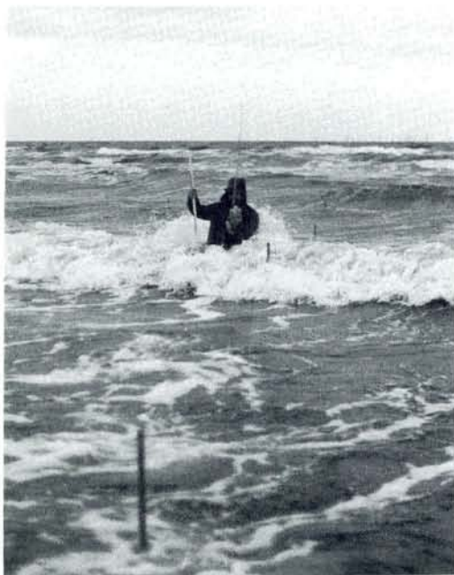
Fig. 6. Measuring in rough weather on 23/9. The permanent pole net makes it possible to take records also under conditions when conventional methods are impossible to use. The single records are transferred to land over the radio.
