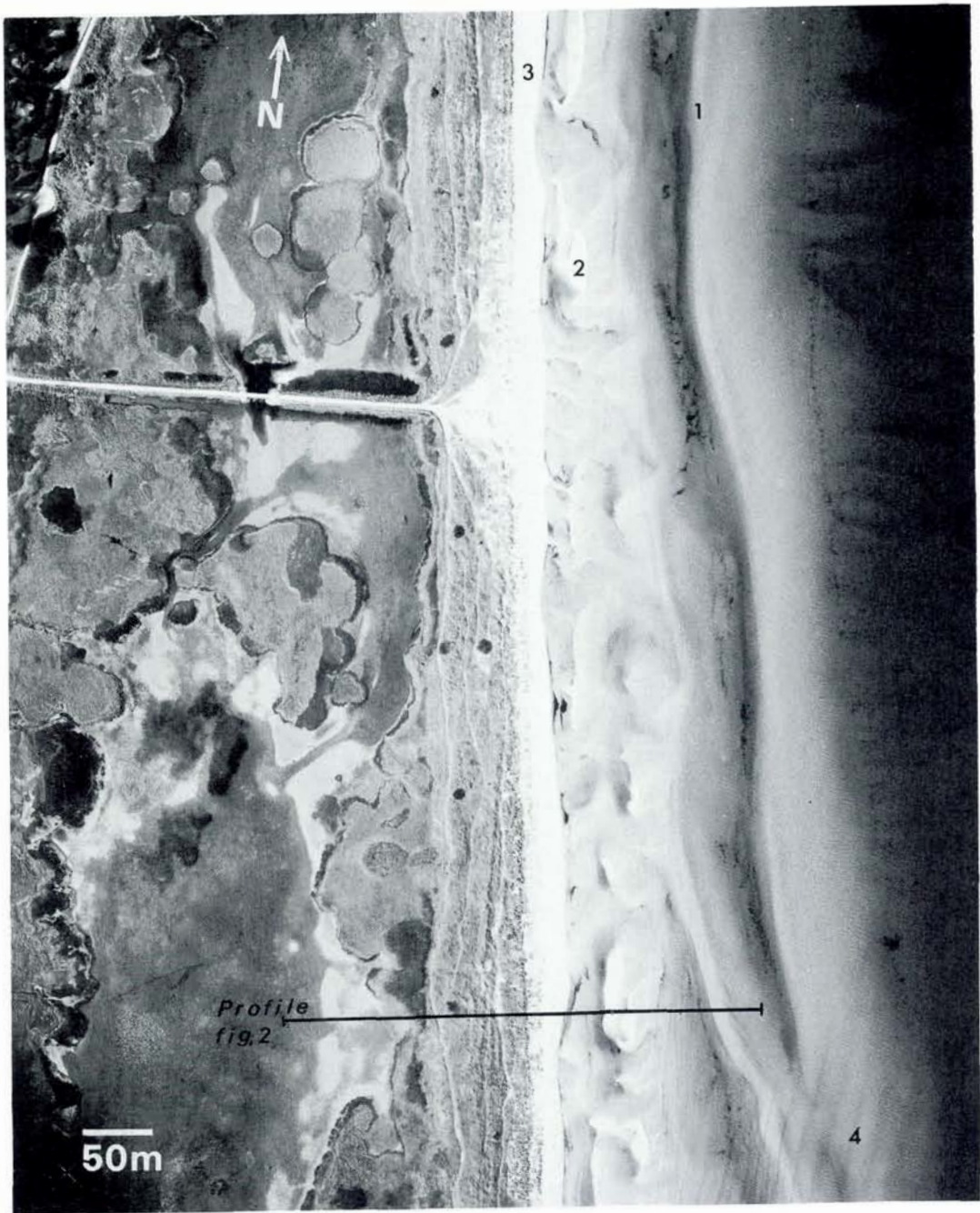
Fig. 3. Part of aerial photograph of Jerse Strand from 21/4 1971. The profile line from fig. 2 is inserted and shows the northern border of the study area. 1. breakpoint bar; 2. near-shore bar; 3. beach and 4. swells. (Air photo: LLO).
