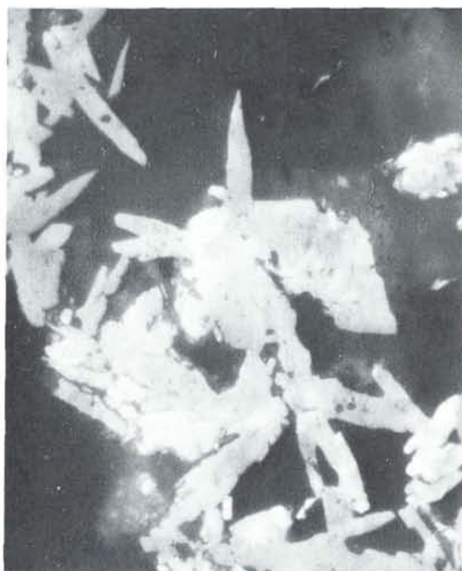
Fig. 7. Polariser only, \times 800 oil immersion. Idiomorphic anatase. Polished section of concentrate of sample 33014 from Gadeby quarry.
