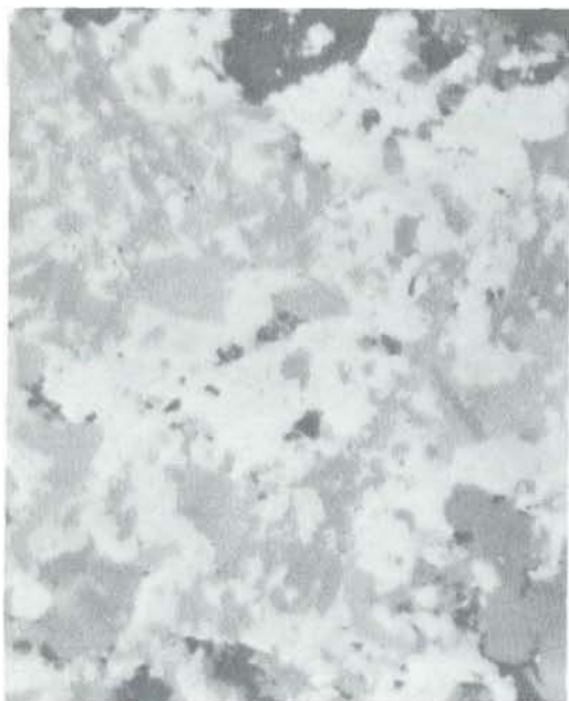
Fig. 6. Polariser only, \times 800 , oil immersion. Hematite-rutile intergrowth. Polished section of concentrate of sample 33015 from Gadeby quarry.
