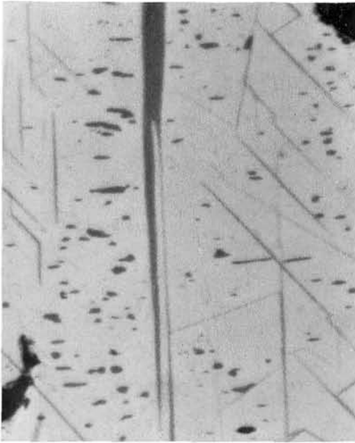
Fig. 2. Polariser only, \times 800 , oil immersion. Hematite-rich ilmenite-hematite exsolution intergrowth with lamellae of rutile. Polished section of concentrate of sample 33014 from Gadeby quarry.
