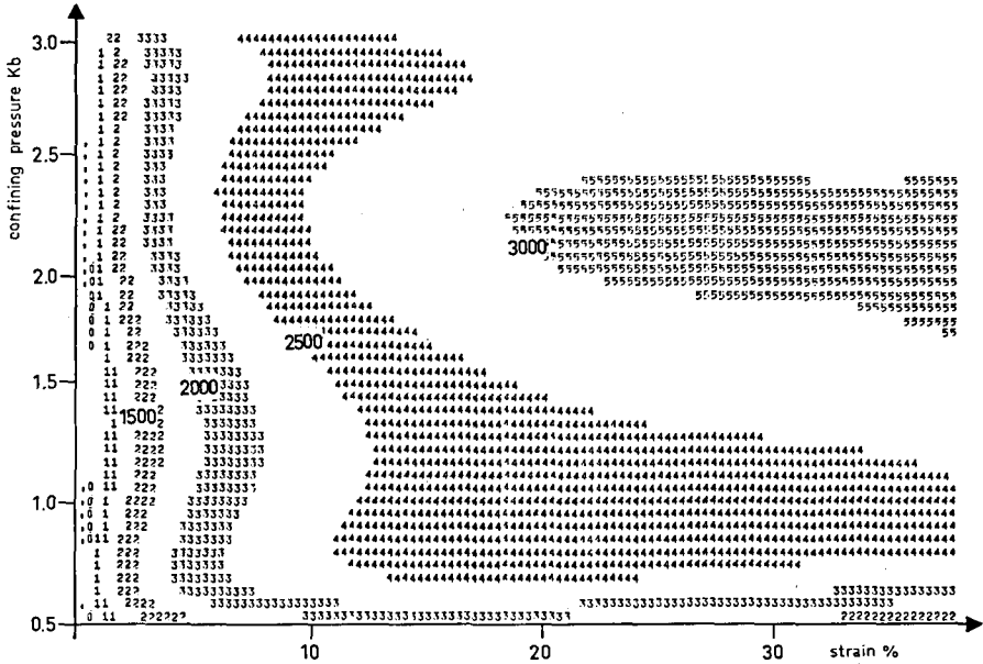
Fig. 11. Contoured surface of the strength of galena of the series LGA 2 dependent on strain (x) and confining pressure (y) computed by stepwise regression from 6 mean stress-strain curves.
