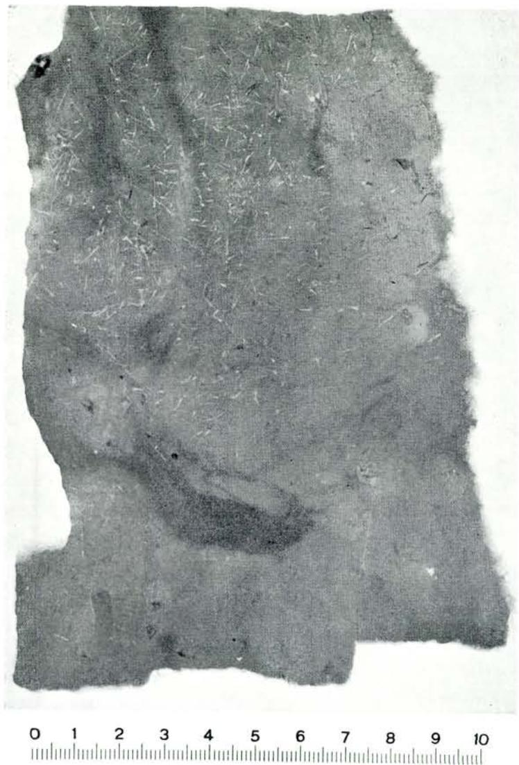
Fig. 9. White chalk, Aalborg. Radiograph. Thickness of slice: 4.0 mm. Film: Ilford Ilfex. kV: 35. mA: 5. Time of exposure: 30 seconds.
