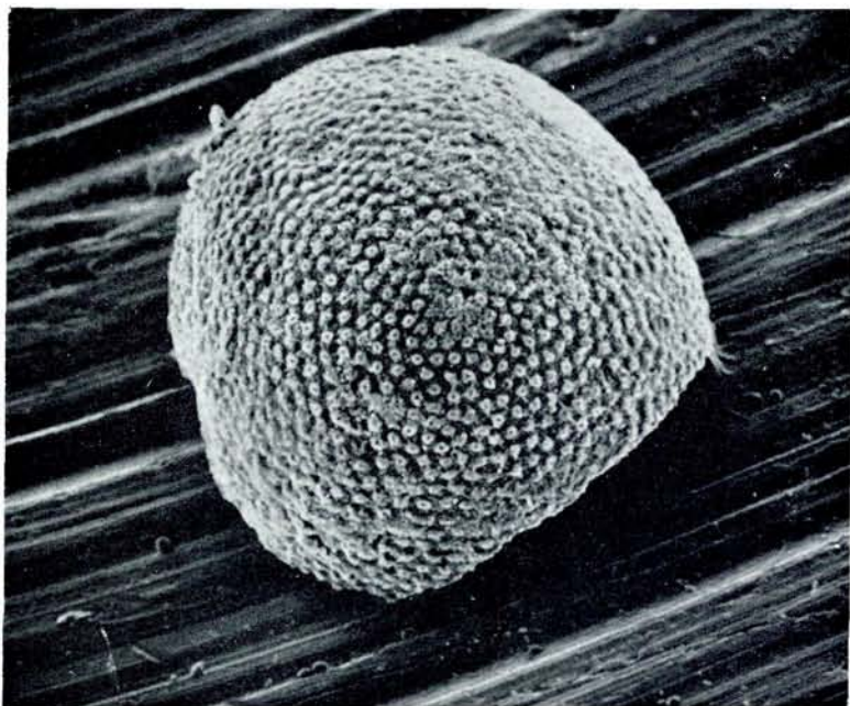
Fig. 2. Surface of a fractured clinoptilolite sphere. Scanning electron micrograph. \times 420 . Locality 3, Rugaard.
