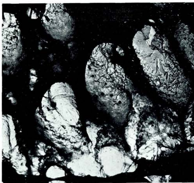
Fig. 2. Detail of interior termination of the channels in a clinoptilolite sphere. Electron micrograph of a two-stage replica. \times 9000 . Locality 3, Rugaard.
