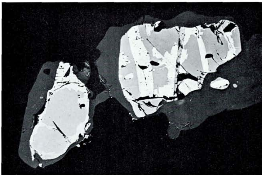
Fig. 1. Polariser only. \times 150 . Oil immersion. Hammer granite (Hammeren). Martitised magnetite surrounded by a broad rim of sphene. The magnetite contains an ilmenite lamella which shows alteration to sphene (almost black) as well as alteration to hematite and rutile.
