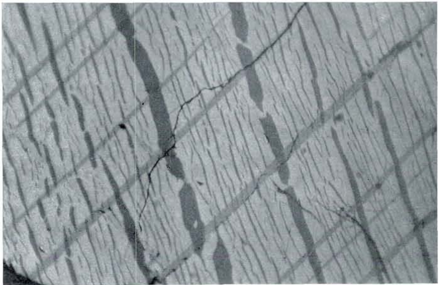
Fig. 2. Polariser only. \times 720 . Oil immersion. Ilmenite-hematite exsolution intergrowth with polysynthetic lamellar twins.
