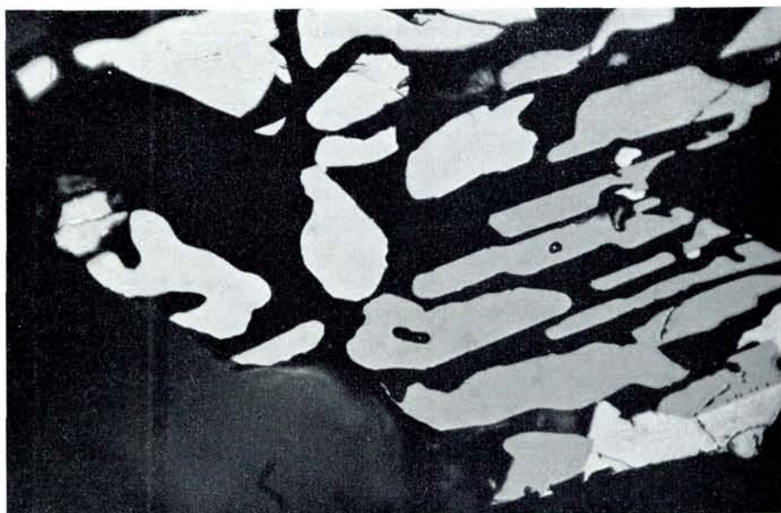
Fig. 1. Polariser only. \times 720 . Oil immersion. Myrmekitic intergrowth of ilmenite and silicates. In the lower right corner some heterogeneous magnetite is intergrown with the ilmenite.
