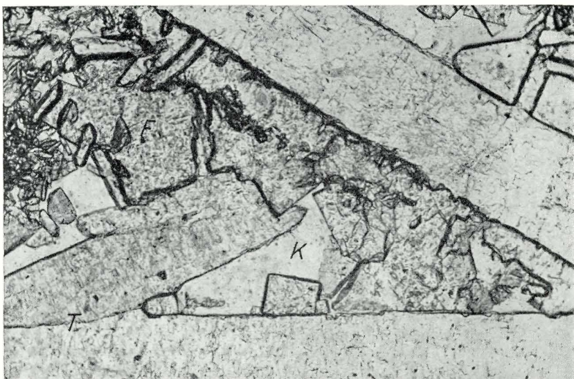
E. Poulsen, fot. Fig. 7. Tungspathjergart (199. 3. a.B.), Vidauban, S. Frankrig. || Nic. \times 100 . T = tungspat; F = flusspat; K = kvarts. Barite rock, Vidauban, Southern France. T = barite; F = flusspar; K = quartz.
