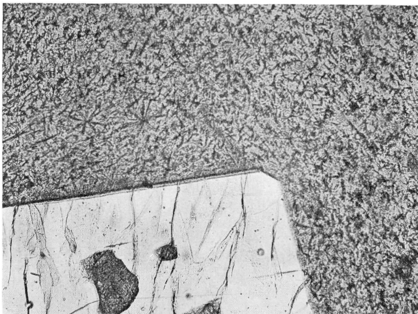
Fig: 3. Porphyritic obsidian, Kjoárbækur. || Nic. 45 \times . Note stellar arrangements of microlites above big plagioclase phenocryst. CHR. HALKIER phot.
