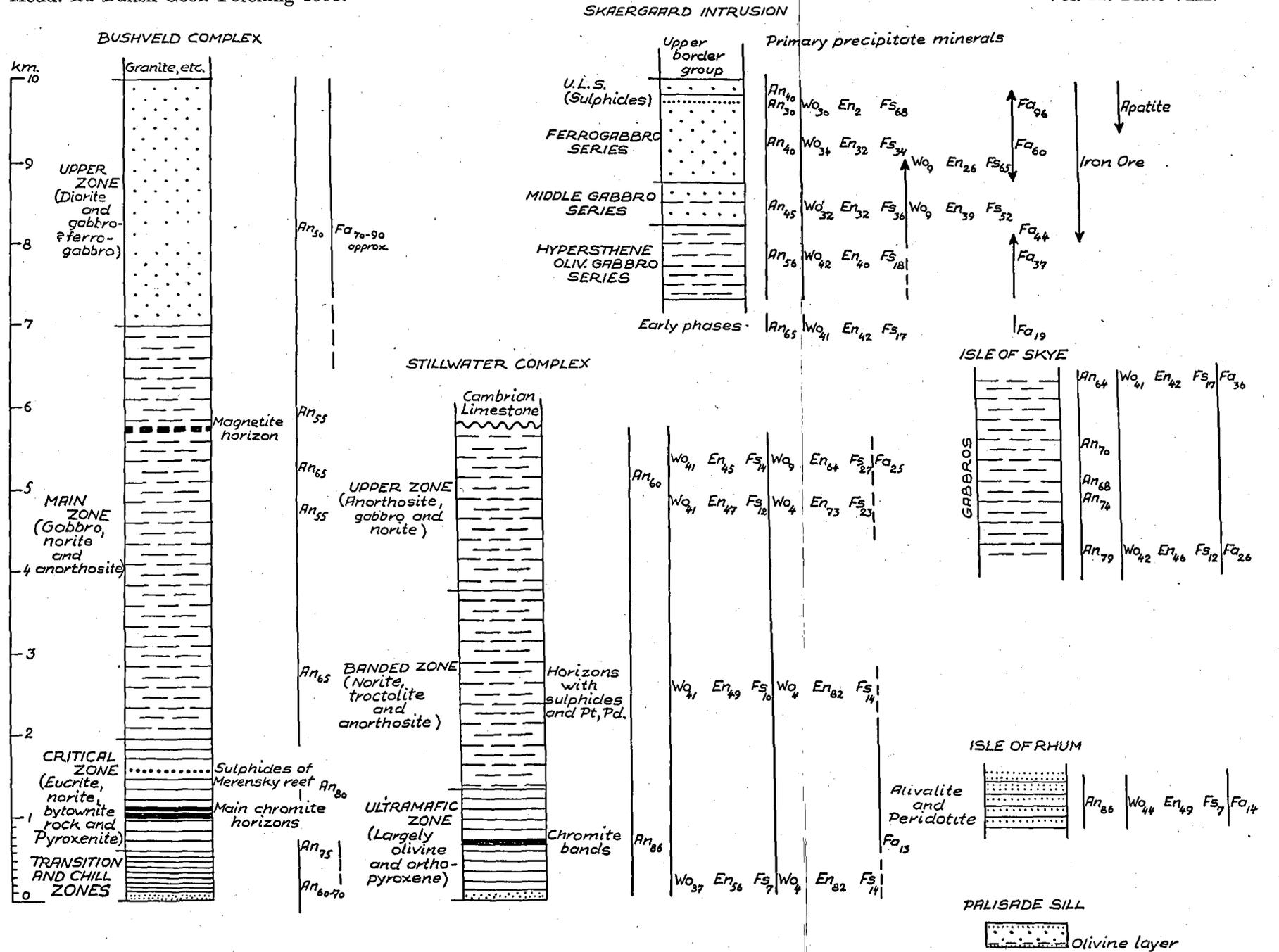
Comparative vertical sections of certain layered intrusions with an indication of the composition of some of the minerals. (Much of the data on thicknesses and mineral compositions are highly generalised).
