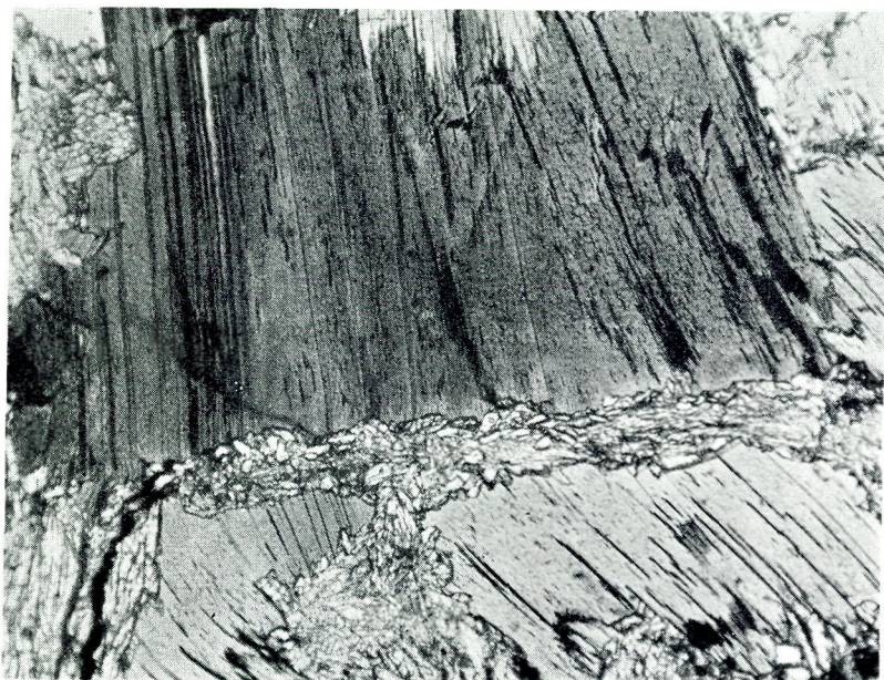
Fig. 2. Pegmatite in Ol_2 (no. 13512). 32\times , 1 nic. A bent and fractured flake of biotite in a matrix of anthophyllite.
