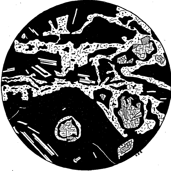
Fig. 6. Peripheral portion of globule, Langesund. Diameter of section: 2 millimeters. Opaque masses are shown in black. Yellowish-brown tachylite with a few slightly anisotropic areas is marked by angle symbols. Yellowish-green devitrified anisotropic glass is shown by ruling. The pyroxenes commonly have opaque mantles. (G. G. U. 36691).
