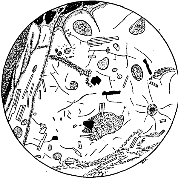
Fig. 8. Peripheral portion of globule, Langesund. Diameter of section: 2.5 millimeters. Showing sideromelane (not marked by symbols) with various alteration products. Along the fissures and in round spots may be seen orange-yellow, anisotropic materials (marked by fine dots). Z symbols : yellow, isotropic material (gel palagonite?). Crescent symbols : reddish-brown, anisotropic, irregularly diffused sections. Cross symbols : green, isotropic material. Gamma symbols : grayish-green, anisotropic material. Angle symbols : green, anisotropic material. Dark areas : almost opaque sections. The stellate mineral in the fourth quadrant is a secondary zeolite. The largest phenocryst consists of augite. In the lower part of the section, beautiful fluidal structures may be seen. (G.G.U. 36694).
