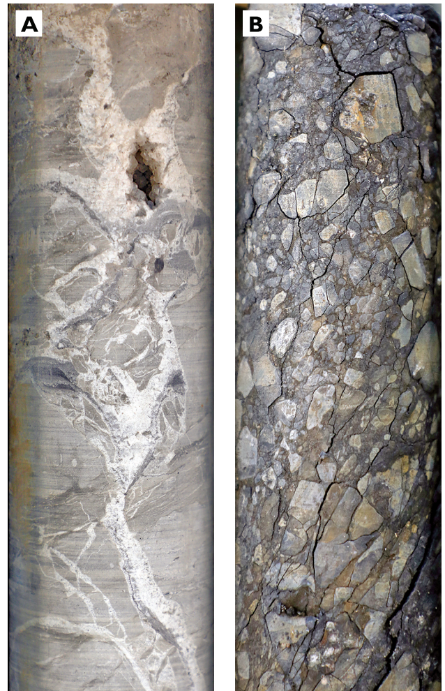
Fig. 5. Breccias in the 55 mm wide Hjulmagergård-1 core. A. Crushed and re-cemented Komstad Limestone, 15.45–15.65 m. B. Crushed Alum Shale, 17.9–18.1 m, photographed in a dry state so that the blackish shale appears grey.
