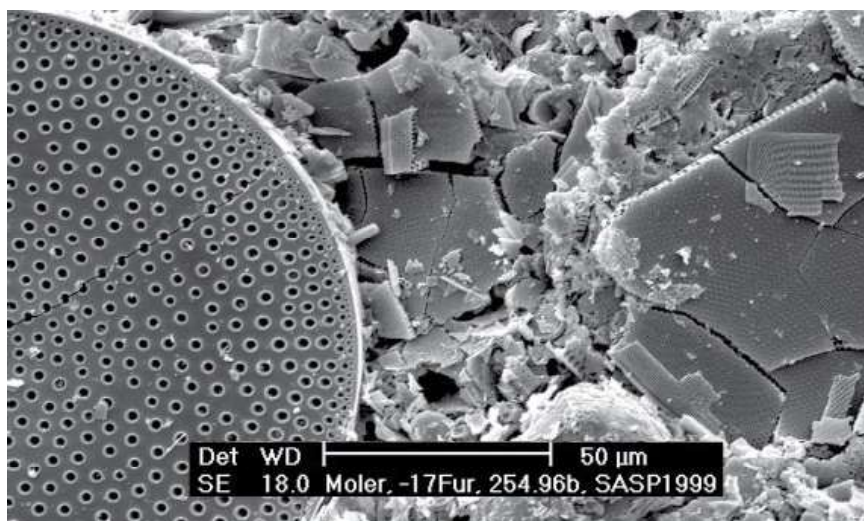
Fig. 4. Diatom frustules with well-preserved fine details, indicating that diagenetic alterations were minimal. SEM photomicrograph of sample stratigraphically below 115.
