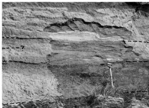
Fig. 8. Debris flows containing streaks, lenses and interflow alluvial sands. There are a minimum of 4 flows and possibly as many as 6 in this section. The flows coarsen upwards and the lower two flows are quite clayey in character. Note the overturned layer of alluvial sand and stretched out and folded fragment of sand (just above shovel handle), all of which indicate flow from left to right (north to south). Location is near Lyngby, Jutland, Denmark.
