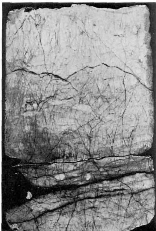
Fig. 15. Valhall Field. Better reservoir quality rock consisting of a lag of chalk pebbles and heavier grains.
