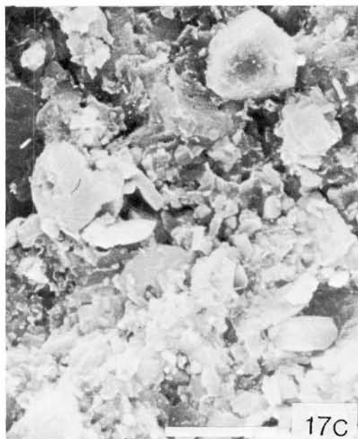
Fig. 17. Scanning electron micrographs of rock types from Valhall Field (after Hardman and Eynon 1977). These types refer to figure 20. Note the corrosion of the coccolith fragments in type A, the overgrowths on the coccoliths in types B and C and the clay minerals in types C and D. Average
