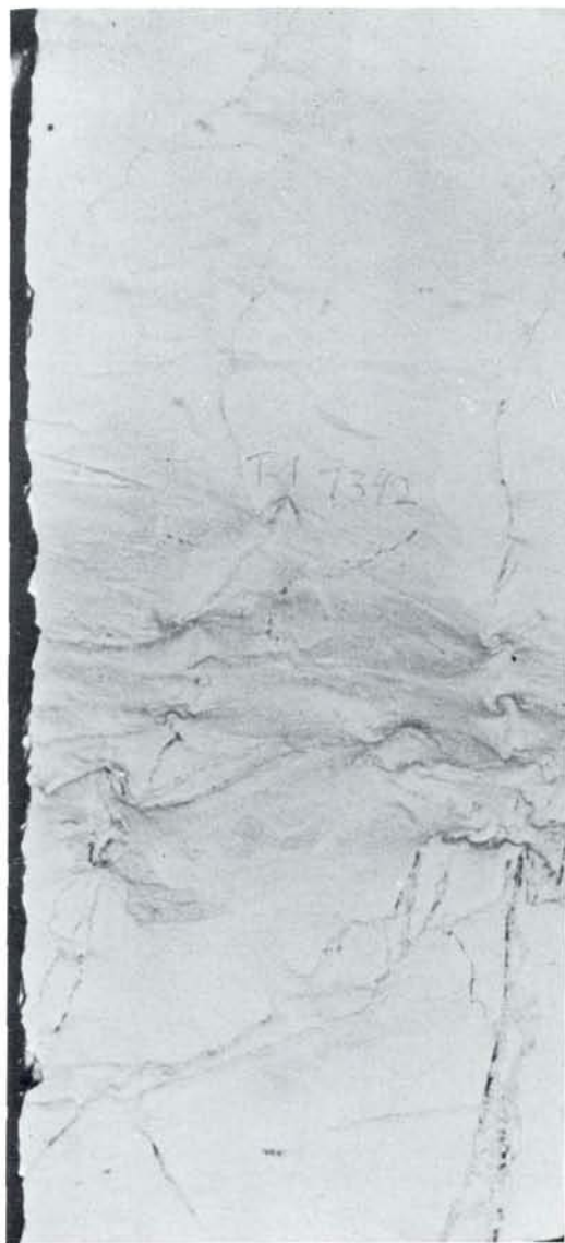
Fig. 16. Evidence that an early rigid framework does not form in clay-rich chalks. Fractures, one of which is clearly seen on the right-hand side of the photograph, are transformed into a zone of isoclinal folding in the clay rich middle part of the core. Having passed through this zone, fracturing is resumed. The specimen is from the Ekofisk Formation of well T-1 in Danish waters.
