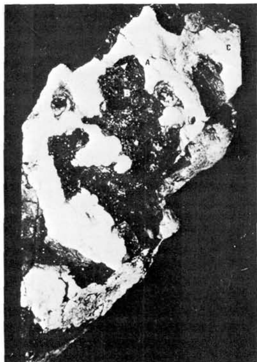
Fig. 14. A highly burrowed chalk from well 2/11-3A Hod Field. The matrix is well cemented, but the burrow fill is much more porous and oil stained. The rock is transitional to a hard ground.
