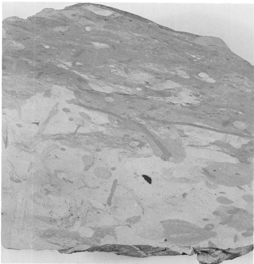
Fig. 3. As fig. 1, but photographed dry by ultraviolet radiation using a Wratten 2E total UV filter. The UV source was an Osira 80 watt mercury bulb having a Wood's Glass envelope, transmitting 95% 3650 Å. \times 1 .
