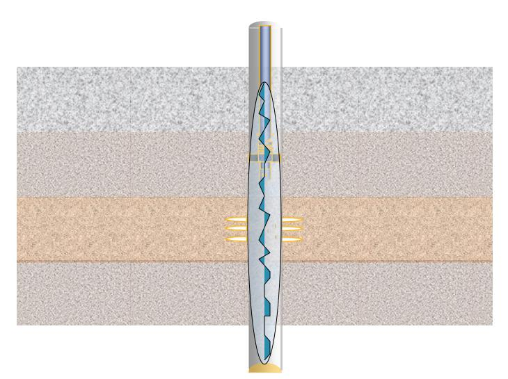
Etched faces of the fracture walls come together unevenly, creating an open pathway to the wellbore.
