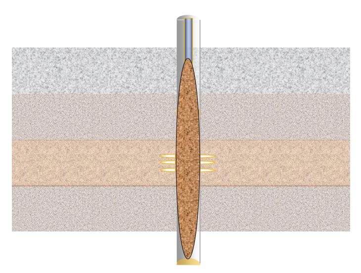
Fracture is packed with proppant, creating a conductive pathway or wick to the wellbore.
