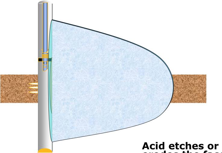
Acid etches or erodes the faces of the fracture
